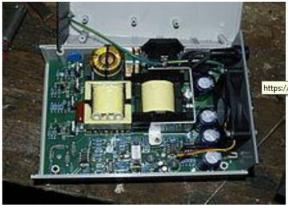
Fig2. Inside of a SWEA 250W Transformer-based grid-tie inverter.
