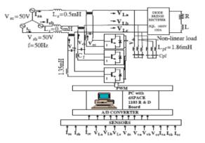
Fig 1. Schematic diagram of the control and power circuit of the HSAPF.
