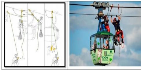
Picture: 2 Descent of the victim through the "Petzl" system
