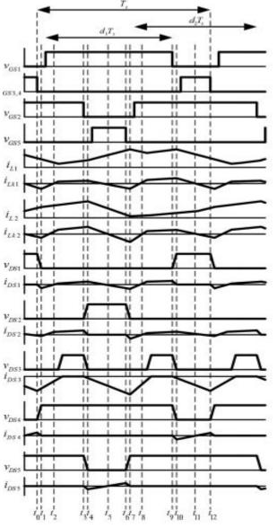
Fig 4.3.Key waveforms of the designed converter.
