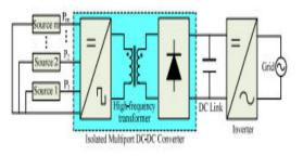
Fig. 1.Configuration of a two-stage, gridconnected, multisource energy system.
