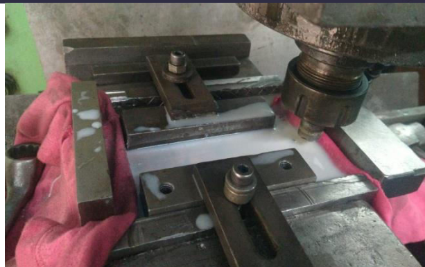
Fig-5: Maintaining 5mm water level above the plates to be welded.
