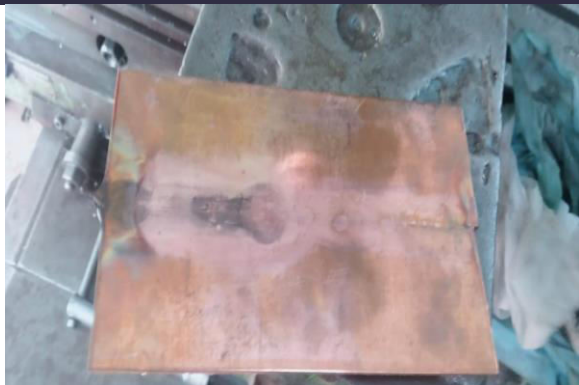
Fig-6: pieces after welding (front portion).
