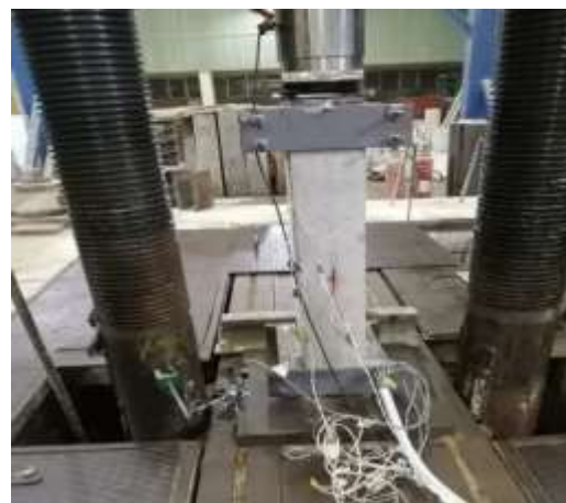
Figure 1.9: BFRP Column tested under axial load.
