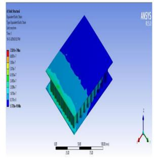
Equivalent elastic strain for aluminium
