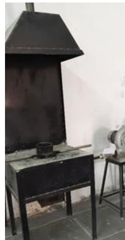
Fig-6: OPEN FIREPLACE FURNACE
