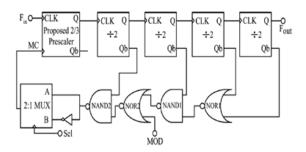
Fig.3.2.Block diagram of 32/33 and 47/48 modes.
