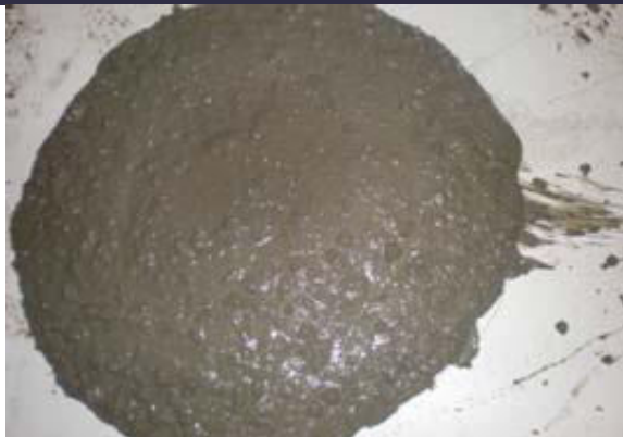
Fig.3.1. Self-consolidating concrete using metakaolin.
