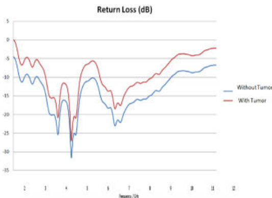
Fig. 5. Return loss (dB) due to antenna on brain phantom(jeans)
