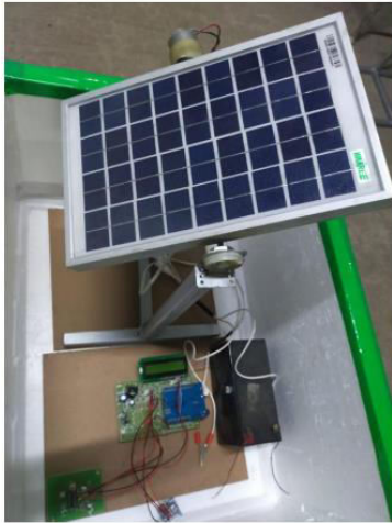
Fig 5.6.3 Hardware setup developed with dual axis tracking Solar panel with floating bed
