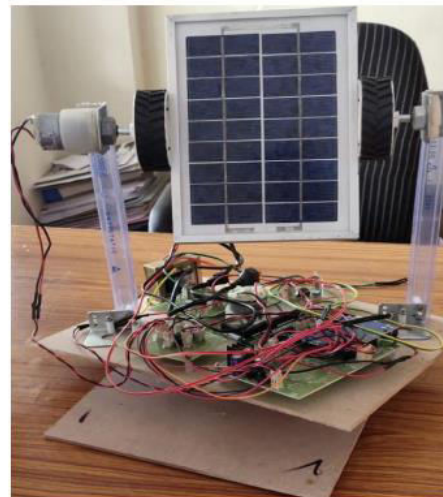
Fig 5.6.2 Hardware setup developed with dual axis tracking Solar panel
