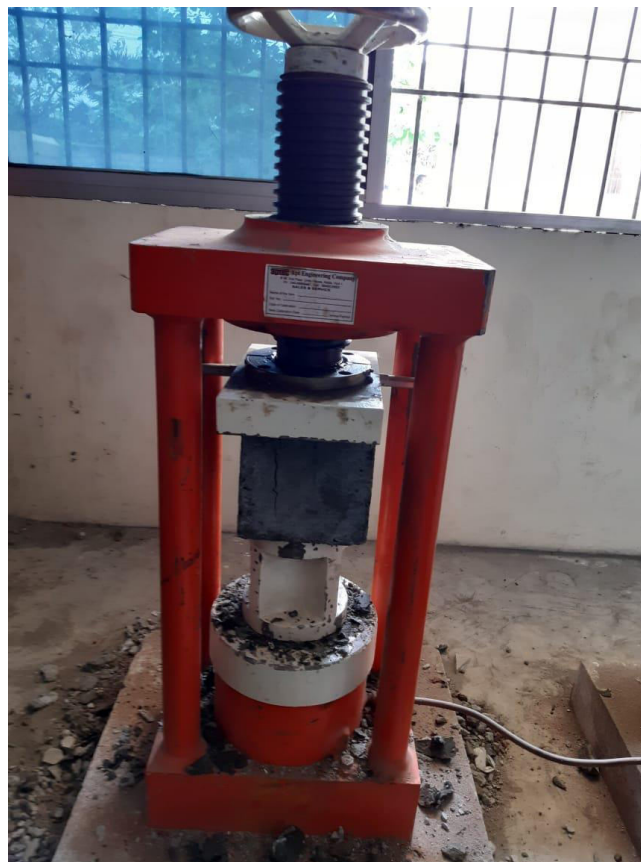
Fig. 2: Compressive strength testing machine.
