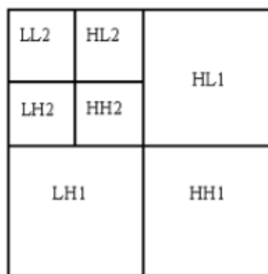
Fig 3: Two level DWT decomposition of an image
