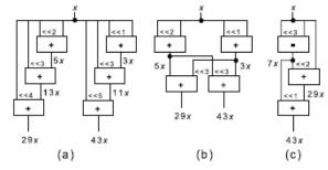
Fig. 2. Shift-adds implementations of 29*x* and 43*x*. (a) Without partial product sharing [2] and with partial product sharing. (b) Exact CSE algorithm [5]. (c) Exact GB algorithm [6].
