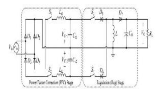
In this section, a high-frequency-fed ac-dc power converter is presented as given in Figure 3 and its operating and control principles are explained The advantageous features of this converter include near-unity input power factor and only one switching action per cycle for all the power switches.
