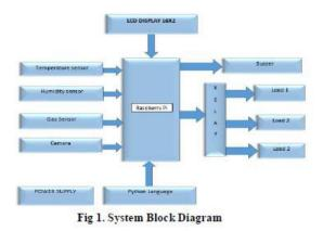
Here Raspberry Pi will be connected to the Wifi which will send these images over the Internet by which the user will be able to see the images and can keep a watch on proper opearation of his system.
