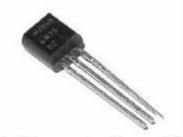
Fig 3. Temperature Sensor LM35
