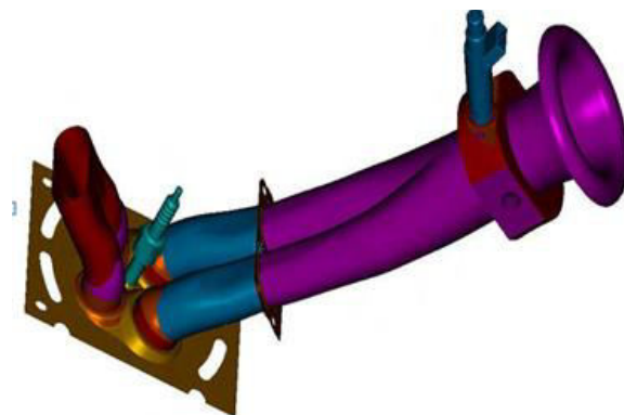
Fig : CAD image of the downdraft intake duct for the W-9 engine.
