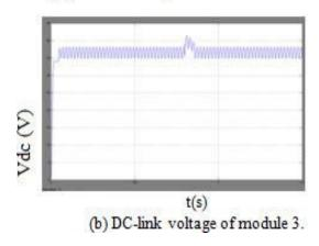
Fig.6. DC-link voltages of phase a with distributed MPPT (25.C)
