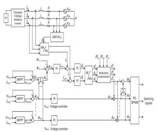
Fig. 3. Control scheme for three-phase modular cascaded H-bridge multilevel PV inverter
