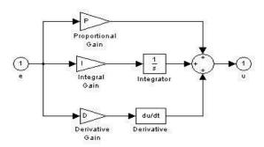
Figure 5. Simulation model of PID Controller
