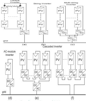
Fig.1. Configurations of PV systems. (a)
