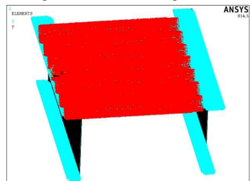
Fig: shows the boundary conditions of the model
