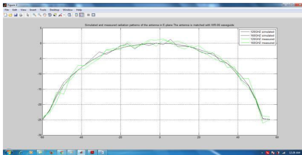
FIG: Simulated and measured radiation patterns of the antenna in E-plane. The antenna is matched with WR-06 waveguide
