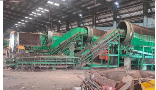
Fig: Monsoon Section/Coarse Segregation 3.0 WASTE TO ENERGY:
