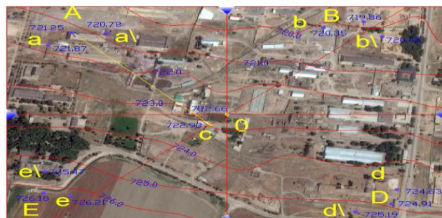
Figure 1. Image of detection of point distortion under the influence of relief in aerial photography.
