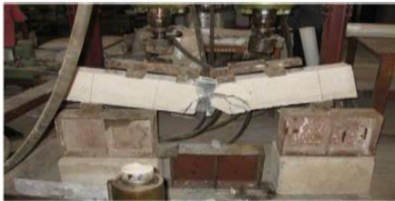
Fig. 5.20 Failure of beam CB1
