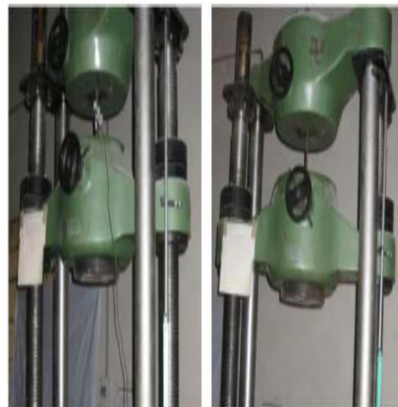
Fig. 6 Tensile Strength of Steel in Electronic UTM
