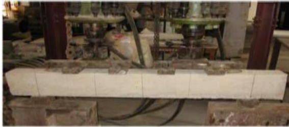
Fig 10 Loading arrangement beam CB1
