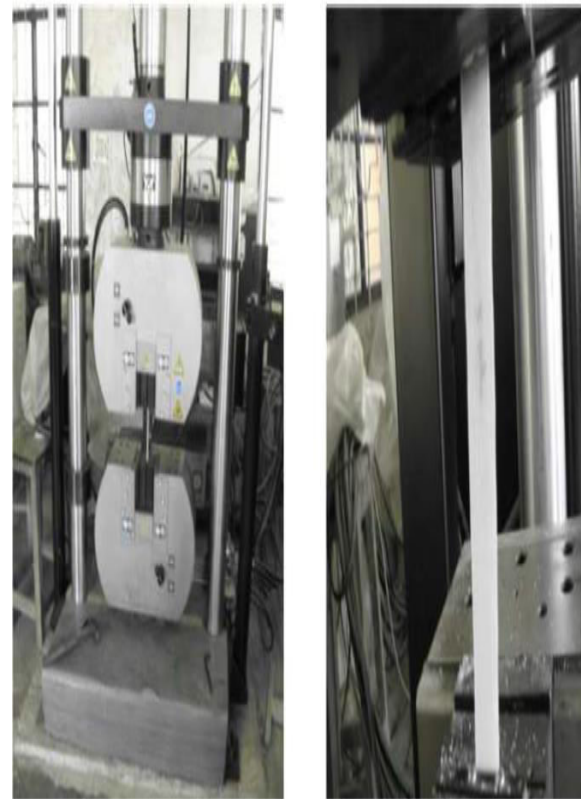
Fig.7 Test of FRP plate in INSTRON 1195
