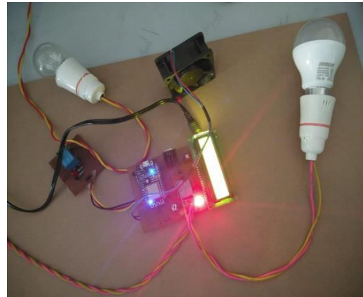
Fig 12 : Fan Turned ON
