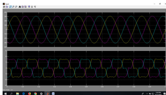
Fig.4.2. Grid side voltage and current.
