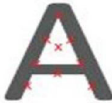
Fig.5. some invariant points (red crosses) of "A". Clickable points in TextPoints are salient points of their characters and thus help remember a password, but cannot be
