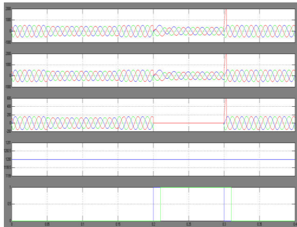
Fig.14 Forward switching simulations of the MCDVR system, top to bottom : (a) the load current, (b) the current in the thyristor's path, (c) the output current of the VSI, (d) the dc-link voltage, and (e) the timing sequence.
