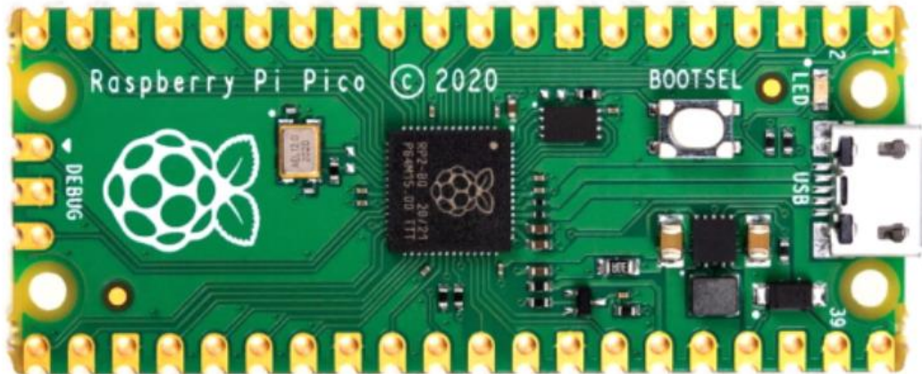
Fig. 3: RASPBERRY PI PICO Development Board.
