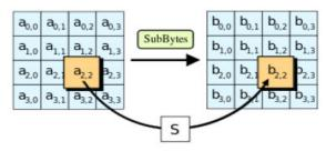
FIG.3. Diagram of Sub Bytes
