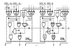
FIG.2. Carry Full Adder Circuit
