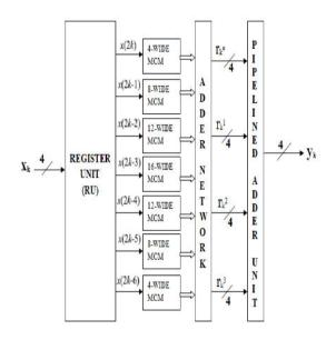
Fig. 2 Proposed structure for fixed FIR filter using MCM
