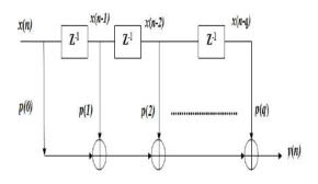
Fig. 1 Finite Impulse Response Filter Realization
