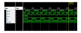
Fig. 7 Simulation Result of : Manchester Encoding
