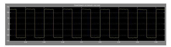
Fig 5.Transformer secondary voltage
