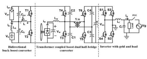
Fig 1.Circuit Diagram of Proposed system
