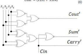
Fig.2. Gate Level Design Approximate Compressor Desin1
