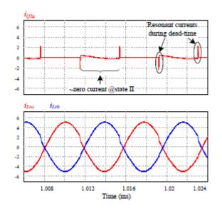
Fig. 9. Zero current characteristic of *Q*2a.
