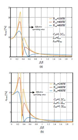
Fig. 8. Current error between the phases as a function of the switching frequency for: (a) Crb=1.2Cra, (b) worst case component's mismatch: Crb=1.2Cra, Lrb=1.2Lra, Lmb=1.2Lma.
