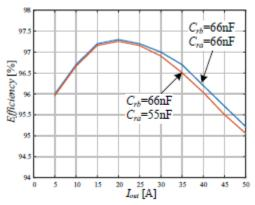
Fig. 16. Efficiency measurements of the experimental prototype.
