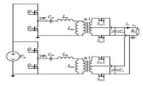
Fig. 2. Conventional two-phase LLC converter.
