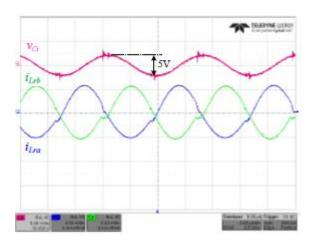
Fig. 13. Experimental waveforms of the TIFLLC converter. C2 – flying-capacitor voltage vCt(5V/div, ac coupled), C3 – phase a primary-side resonant tank current *iLra*(5A/div), C4 – phase b primary-side resonant tank current *iLrb*(5A/div). Time scale is 2µs/div.
