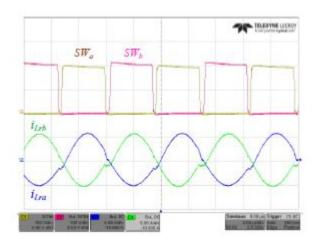
Fig. 14. Experimental waveforms of the TIFLLC converter. C1 – switching node voltage of phase *a SWa*(100V/div), C2 – switching node voltage of phase *b SWb*(100V/div), C3 – phase *a* primary-side resonant tank current *iLra*(5A/div), C4 –
