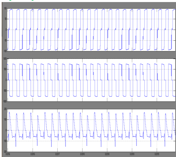
Fig 5 Simulation wave form of the line voltage V_{AB} across the primary and secondary of the transformer and the line current I_{lk1}
