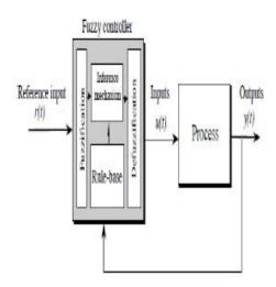
Fig.4. General Structure of the fuzzy logic controller on closed-loop system
