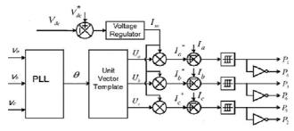
Fig. 2. Block diagram representation of gridinterfacing inverter control.
