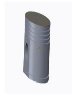
Fig 3.3: Ceramic coated piston with 0.4mm coating layer
