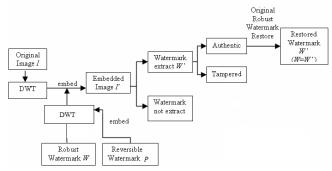
Figure 3. A block diagram for meddle watermarking
