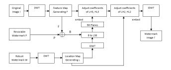
Figure 4.A block diagram for Watermark Embedding
