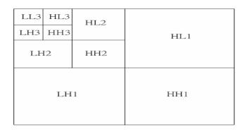
Figure 2.Shows illustration of Wavelet Decomposition
