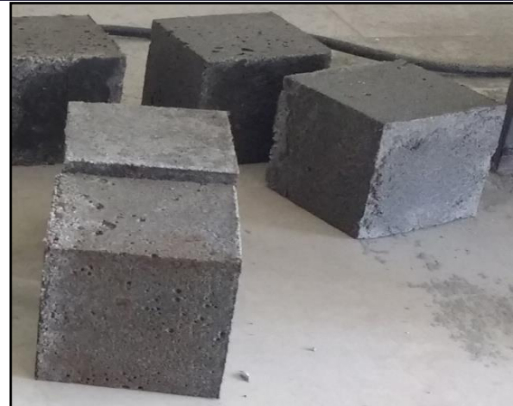
Fig. 1: Test specimens for compressive strength
