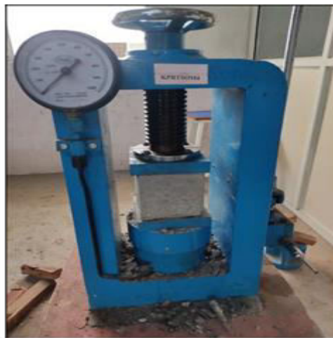
Fig. 13: Testing of Cube Specimen.
