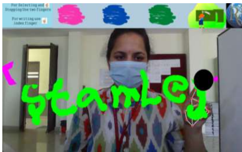
Fig 15 Realtime Finger Writing Recognition Using Web camera -It is a effective interface where a user can directly write and erase the content on the screen. This image demonstrate how do we erase the content on the screen for doing that we need first select the erase button (as symbol is clearly mention on the screen) with 2 fingers(Index and Middle fingers respectively).With one finger we need erase content that is Index Finger.
