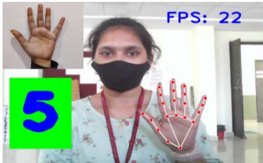
Fig 9 Finger Counting- It is used to detect number of finger that is showed on screen In this image it demonstrate the count of five
