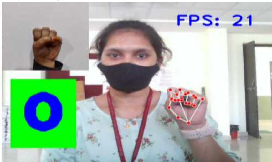
Fig 4 Finger Counting - It is used to detect number of finger that is showed on screen In this image it demonstrate the count of zero
