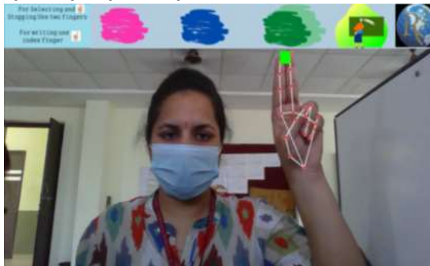
Fig 12 Realtme Finger Writing Recognition Using Web camera -It is a effective interface where a user can directly write and erase the content on the screen.This image demonstrate how do we select the color-we use 2 fingers(Index and Middle Finger) for selecting.
