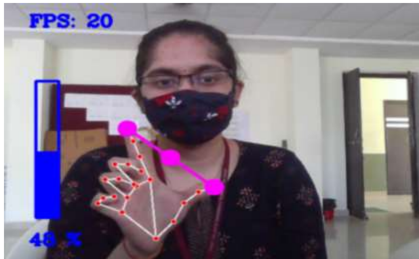
Fig 11 Volume Gesture -This application works when your trying stretch with 2 fingers. This image demonstrate the medium stretch percentage i.e 45%.
