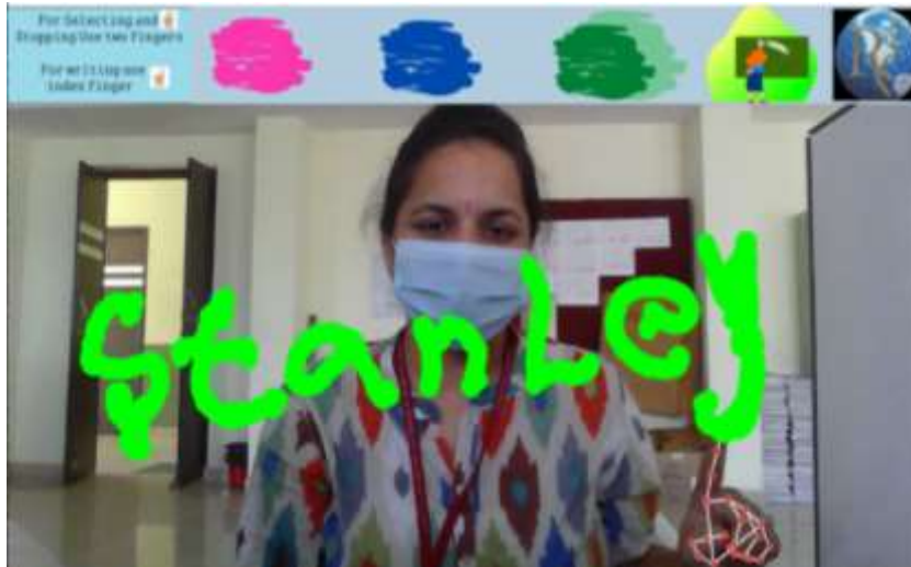
Fig 13 Realtime Finger Writing Recognition Using Web camera -It is a effective interface where a user can directly write and erase the content on the screen. This image demonstrate how do we write the content on the screen for doing that we use one finger that is the index finger.
