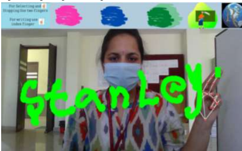
Fig 14 Realtime Finger Writing Recognition Using Web camera -It is a effective interface where a user can directly write and erase the content on the screen. This image demonstrate how do we stop writing on the screen for doing that we use 2 fingers i.e Index and Middle finger respectively.
