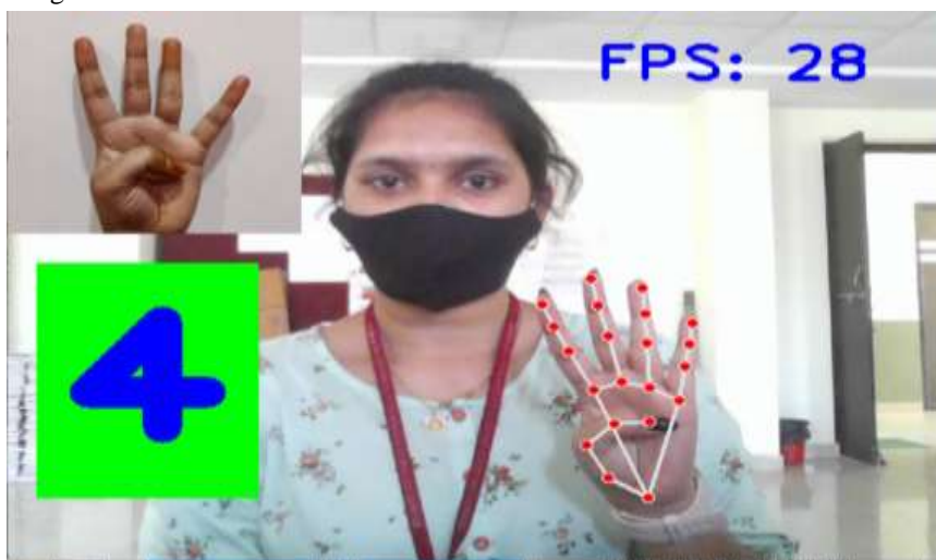
Fig 8 Finger Counting- It is used to detect number of finger that is showed on screen In this image it demonstrate the count of four
