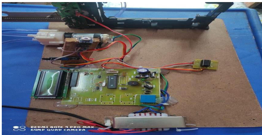
Fig. 6. Automatic Sanitization and Temperature Measure System
