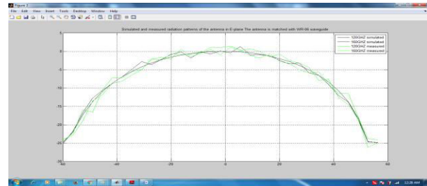
FIG: Simulated and measured radiation patterns of the antenna in E-plane. The antenna is matched with WR-06 waveguide
