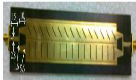
Fig. 8. Photo of the dual elements based LWA antenna prototype.
