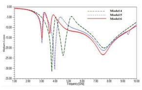
Fig. 2.2 Return Loss for Double Notch
