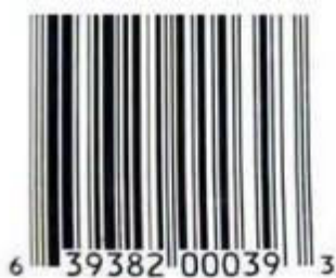
Fig.1. Bar Code Example B. Types of Bar Code 1. 1-D One-Dimensional Barcodes One-dimensional barcode appearance looks
