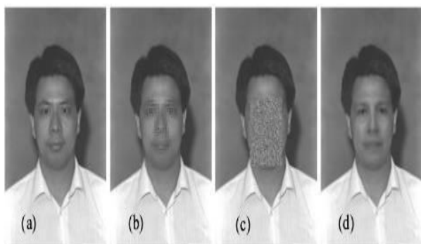
Figure comparing the resulting reversible de-identified images (a) original image, (b) scrambling of DCT coefficients, (c) encryption of pixel values, (d) proposed method
