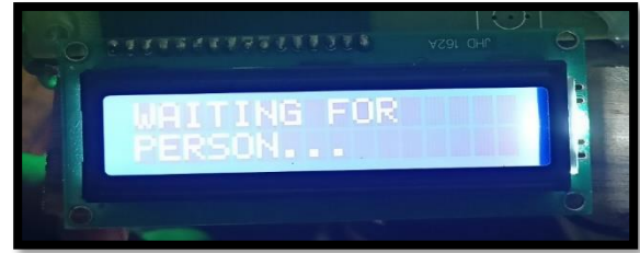
Fig. 6 When the kit detects the person, it checks the temperature and allows the person if he has less than 100°F, a message was pop up as
