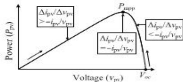
Fig.5. Illustration of INC-MPPT with SPV array  $P_{pv}-V_{pv}$  characteristics.
