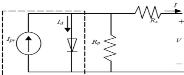
Fig.3. Single Diode Model
