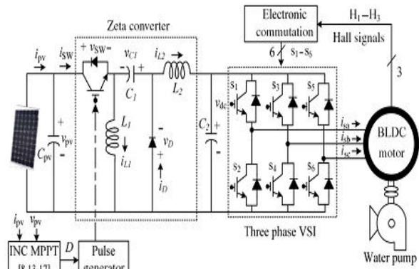
Fig.2. Conventional SPV-zeta converter-fed BLDC motor drive for water pump
