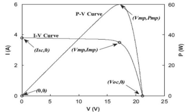
Fig.4. Output characteristics of PV cells
