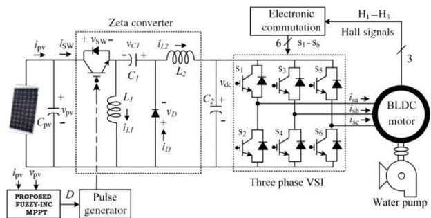
Fig.3. Proposed SPV-zeta converter-fed BLDC motor drive for water pump
